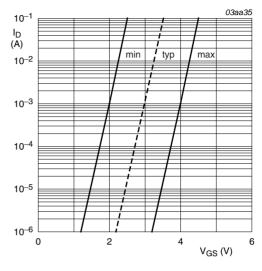
$$T_{j} = 25 \,^{\circ}C; V_{DS} = 5V$$
