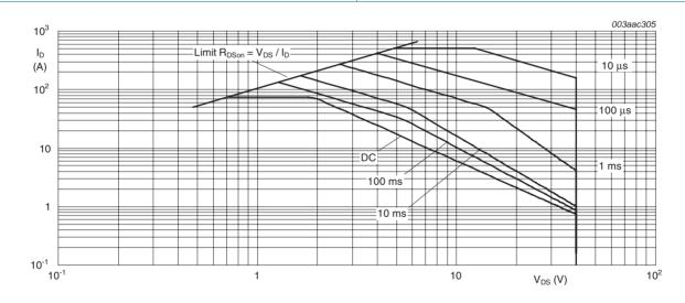
$T_{mb} = 25 \,^{\circ}C; I_{DM}$ is single pulse Capped at 75 A due to package.
