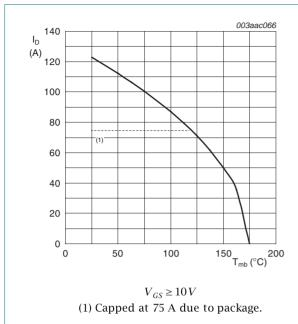
Continuous drain current as a function of mounting base temperature
