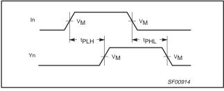
Waveform 1. For non-inverting outputs
