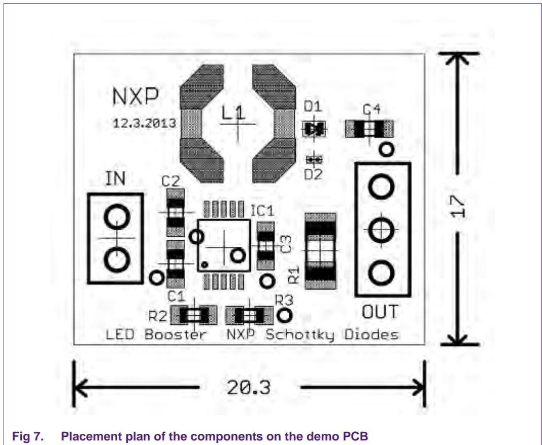
Fig 7. Placement plan of the components on the demo PCB
