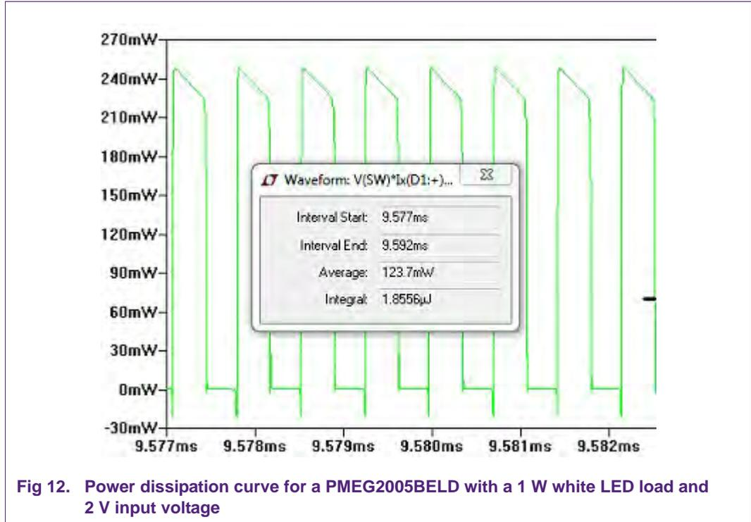
Fig 12. Power dissipation curve for a PMEG2005BELD with a 1 W white LED load and 2 V input voltage
