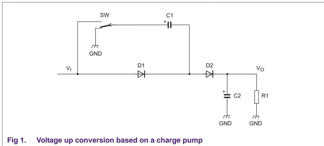
Fig 1. Voltage up conversion based on a charge pump
