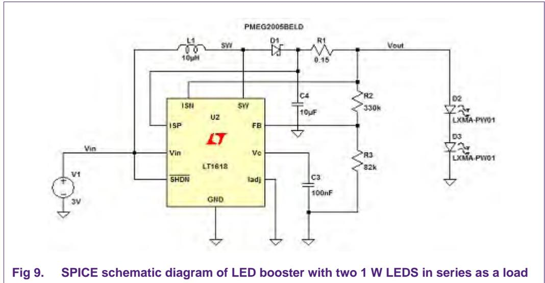
Fig 9. SPICE schematic diagram of LED booster with two 1 W LEDs in series as a load
