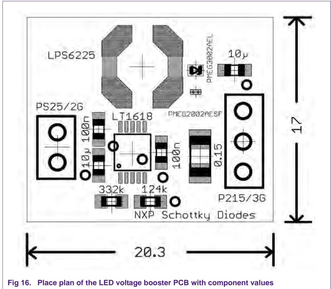
Fig 16. Place plan of the LED voltage booster PCB with component values
