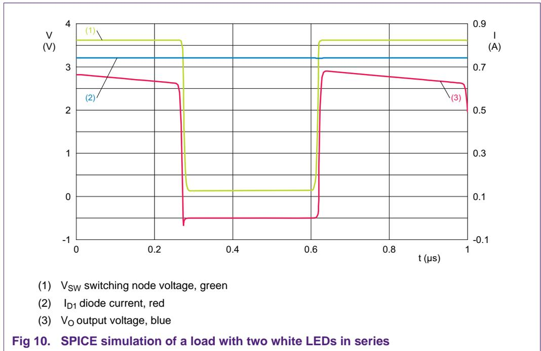
Fig 10. SPICE simulation of a load with two white LEDs in series
