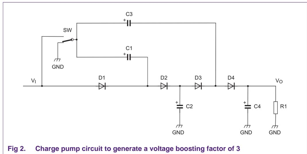
Fig 2. Charge pump circuit to generate a voltage boosting factor of 3
